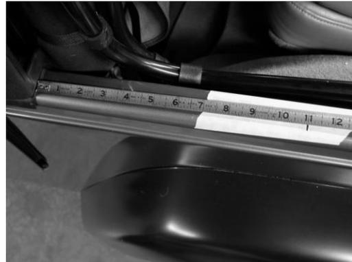
**Step 3:** You will need to mark and drill four holes to install the mounting brackets. Measure from the hole on top of the tub and closest to the door. On our TJ we measured 11" and on our YJ we measured 16". The dimension isn't critical, but it is important to make sure that you avoid the mounting tabs on the driver's side of the tub that are used to hold the wiring harness. It's also a good idea to use the same dimension from one side to the other.
