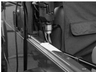
**Step 4:** Take a mounting bracket and place it in position on the tub centered around the mark you made in Step 3.
