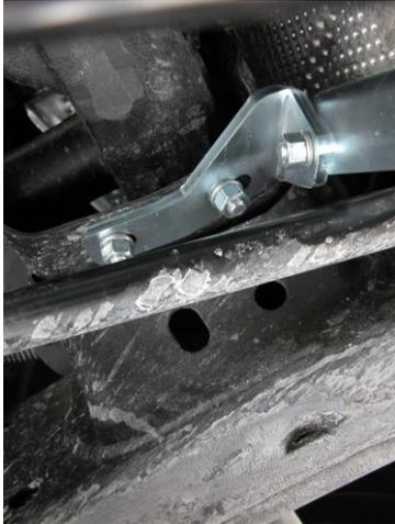
**Step 3:** Install the passenger side-mounting bracket using the bolts just inserted into the motor mount. The mounting tab faces the rear of the vehicle. It is shown with the strut rod attached in the photo to the left. Leave these bolts loose for now.
