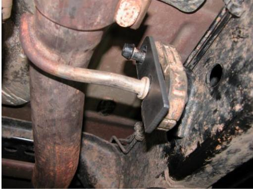
**Step 16:** Place the Exhaust Hanger Adjuster over the exhaust hanger pins as shown in the photo to the left. This “locks” the two pins together to facilitate bending the frame mounted pin upward in the next step.
