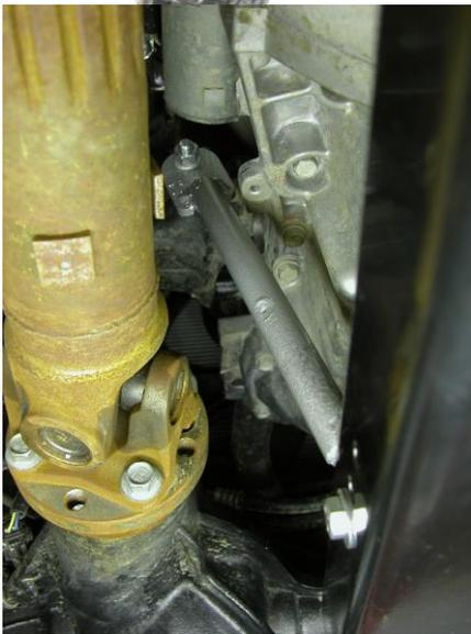
**Step 10:** Install the driver's side strut rod as shown at left, again using one of the 3/8-16 x 1.5" bolts at the top of the strut rod and one 3/8-16 x 1" bolts at the bottom. Make sure to place the strut rod within the skid plate as shown. Also, please note that the strut rod isn't quite symmetrical. It will fit better one way than it does the other, but there is no distinguishing feature for top or bottom.
