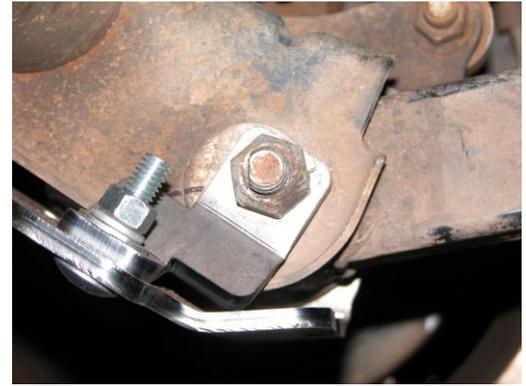
**Step 7:** Bolt the control arm skid plate to the shock mount using the 3/8-16x1" hex head bolts, lock washers, and flat washers. (Driver's side shown below.)
