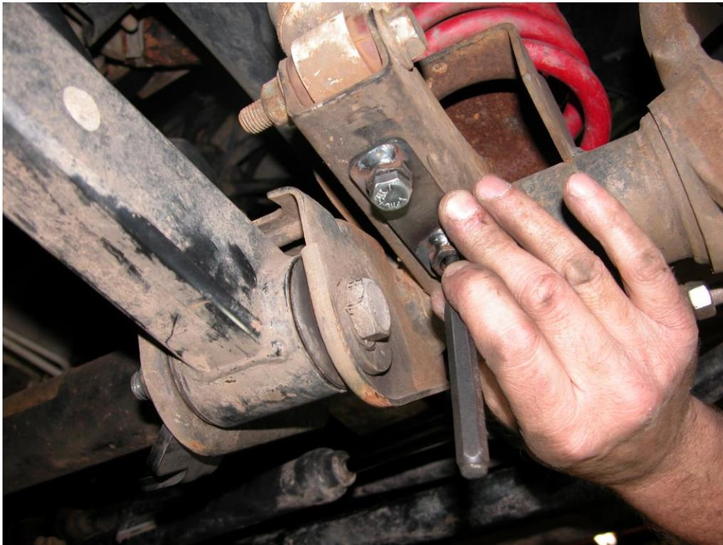
**Step 4:** Remove the nut from the lower control arm bolt. Place the right-side bracket over the control arm bolt as shown in the photo at right. Leave the nut loose at this time.
