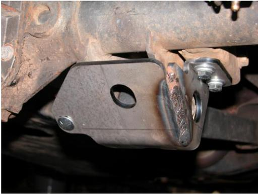
**Step 8:** Once all of the bolts are installed, tighten them. Torque the nut on the lower control arm mounting bolt to the recommended torque. Sorry, but we can't give a number for this since it varies based on model year and whether or not you are using factory or after-market control arms.
